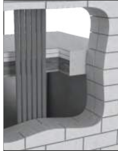
Cut-out for existing cables
